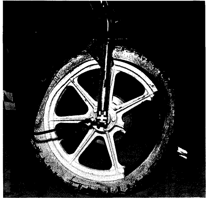
Figure 2. Heavyweight motorcycle cast front wheel after a 13.4 m/s head-on impact
