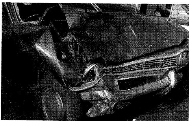
Figure 2. Accident-damaged car showing protruding main box section
