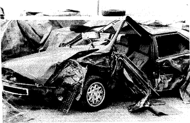
Figure 12. Typical car damage with high offset and extensive intrusion on the left in the area of the driver
