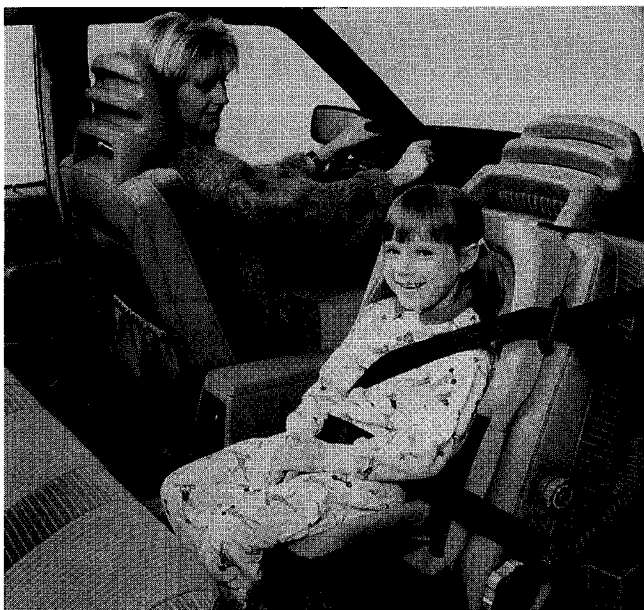
Figure 17. The half-integrated child seat. The child is secured by the front passenger safety belt
