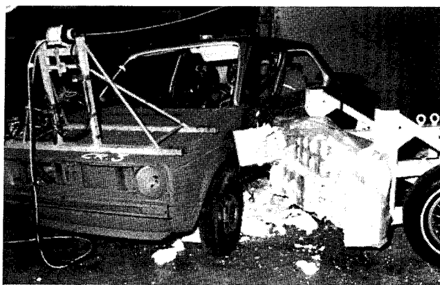
Figure 11. Final position after a collision with the “crabbed” EEVC barrier
