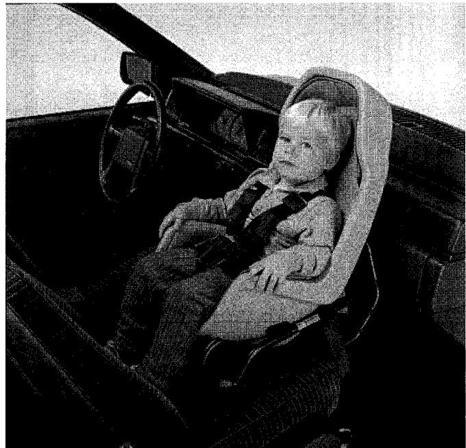
Figure 14. Rearward facing front seat. Infant and toddler position. The child seat is placed on the passenger front seat with its back leaning against the dashboard. It can be adjusted to the desired angle by sliding the front seat forwards or backwards. The child seat is secured by an extra strap together with the passenger safety belt
