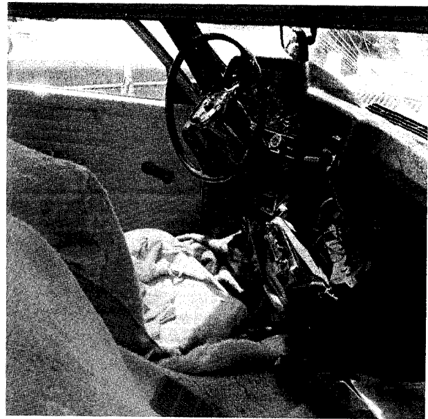
Figure 18. Serious head-on collision with steering column thrust up and into the car
