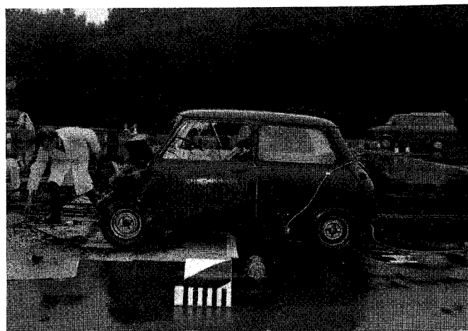
Figure 7. Impact test with truck guard fitted. Truck stationary before impact
