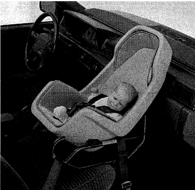
Figure 14. Rearward facing front seat. Infant and toddler position. The child seat is placed on the passenger front seat with its back leaning against the dashboard. It can be adjusted to the desired angle by sliding the front seat forwards or backwards. The child seat is secured by an extra strap together with the passenger safety belt
