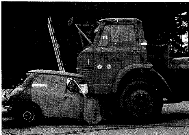
Figure 4. Impact tests without truck guard fitted. Both vehicles moving before impact
