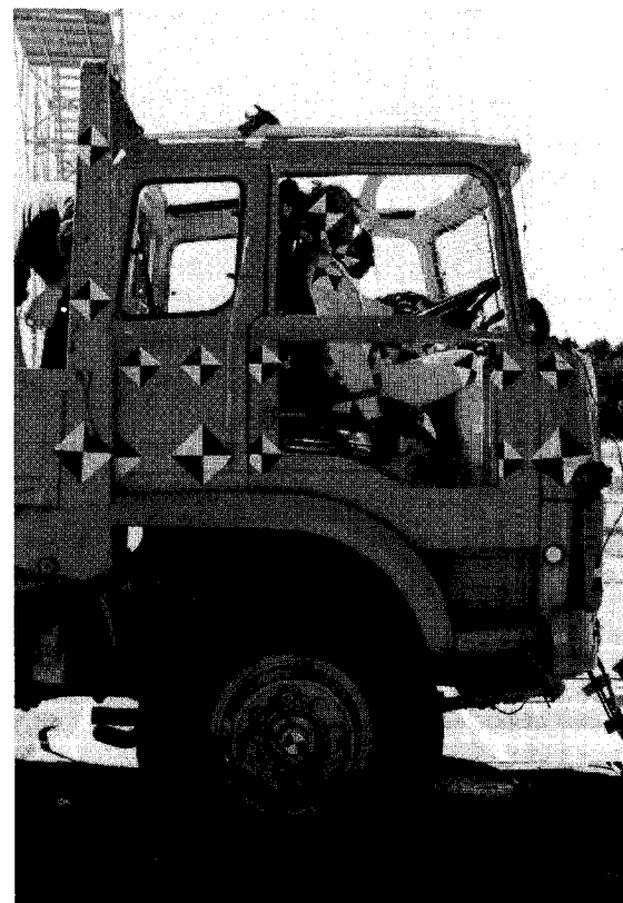
Figure 4. Cab deformation after the test
