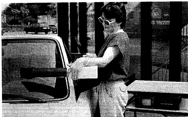
Figure 3. Stray light analyzer for measuring windshield wear in terms of a stray light index.
