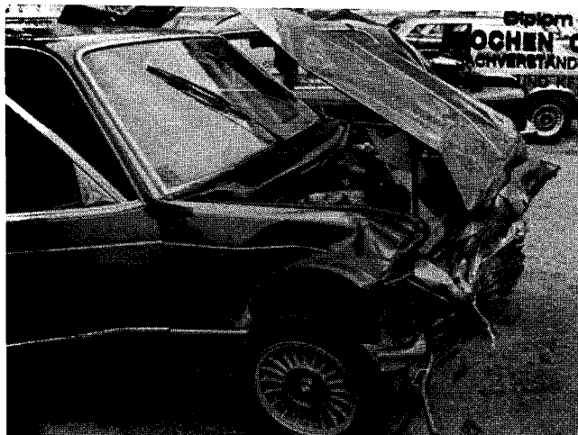
Figure 15. Serious head-on collision with relatively slight injuries to the belted passenger on the left-hand rear-seat
