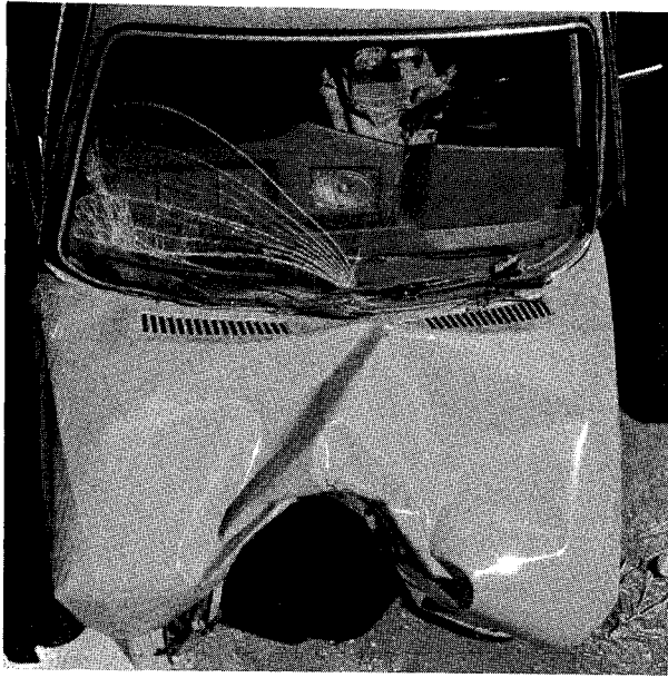
Figure 18. Serious head-on collision with steering column thrust up and into the car
