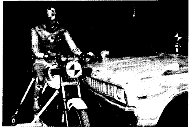
Figure 10. Sled tests set-up for simulated collision
