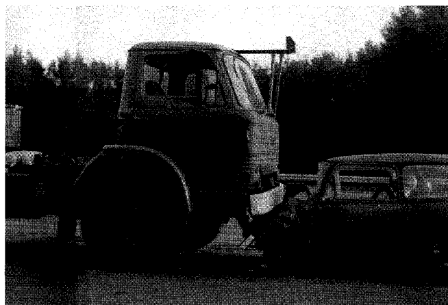
Figure 5. Impact test with truck guard fitted. Both vehicles moving before impact
