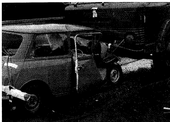
Figure 6. Impact test without truck guard fitted. Truck stationary before impact
