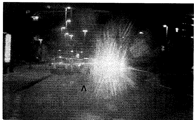
Figure 2. Sight through a worn visor. Both windshields and visors are exposed to the impact of small particles of sand and dust as well as abrasive effects of cleaning efforts. A pedestrian (marked with \wedge ) nearly disappears behind the "tails"
