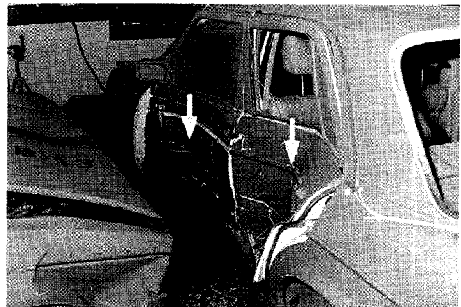
Figure 5. Lateral intrusion VW Golf/DB W 123 (45 km/h)
